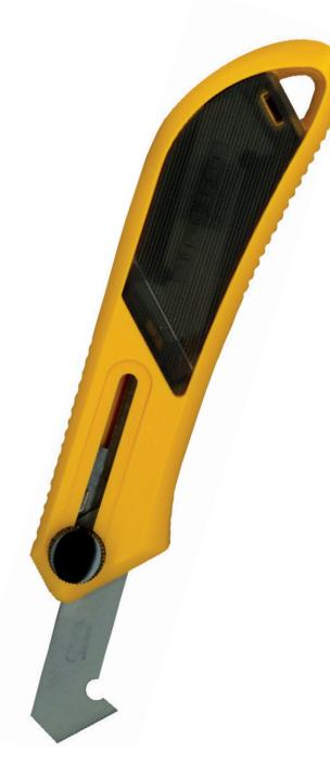
The OLFA® Heavy Duty Laminate Cutter PC-L features a ratchet wheel for secure blade extension and retraction. Sharp and dependable, this tool continues to easily score sheet plastics and laminates to enable the precise breaking of plastic materials. It comes inserted with a reversible tungsten steel PB-800 blade, plus 2 replacement blades tucked in the handle. Uses replacement blades PB-800. Great for cutting plastics and laminates for both construction and industrial applications
